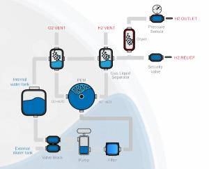
Hydrogen is produced from distilled water using a polymeric membrane (PEM). No acid or alkaline solutions are used.
