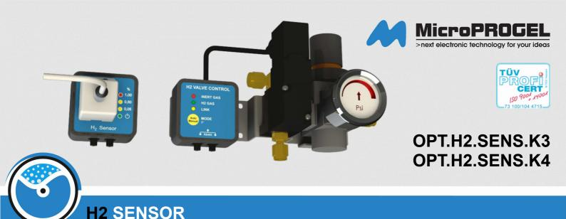
OPT.H2.SENS.2 is a security system that constantly detects the amount of Hydrogen present in the GC's oven and blocks the Hydrogen generation if it detects an amount greater than the safety threshold. The OPT.H2.SENS.RCV controller reads the percentage of Hydrogen measured by the sensor OPT.H2.SENS.2 and, if the value exceeds the threshold alarm, the Controller deactivates the solenoid valve in the OPT.H2.SENS.VB.V2 block.
